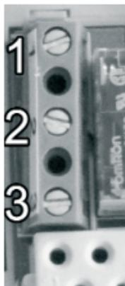
**ATTENTION!** *The device must be installed and connected by a qualified professional. Always follow the manufacturer's instructions when connecting the thermostat to any heating or cooling appliance. The voltage appearing at terminal No. 1, No. 2 or No. 3 depends only on the system being controlled, therefore the dimensions of the wire are determined by the type of the device to be controlled. The length of the wire is of no significance.*
